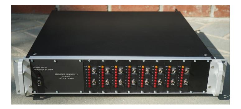
It also has a ninth slot for a user-provided microprocessor which provides gain control outputs, digitizes the preamplifier outputs and communicates via the VME
