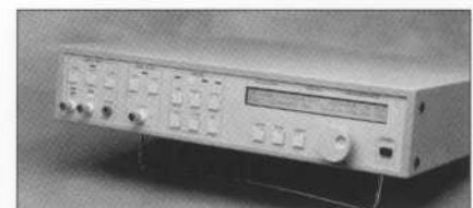
FIGURE 4. Lock-in extender/enhancer operates up to 12.5 MHz and works either as a down-shifting front end to a separate, conventional lock-in, or as a complete, self-contained lock-in amplifier.
